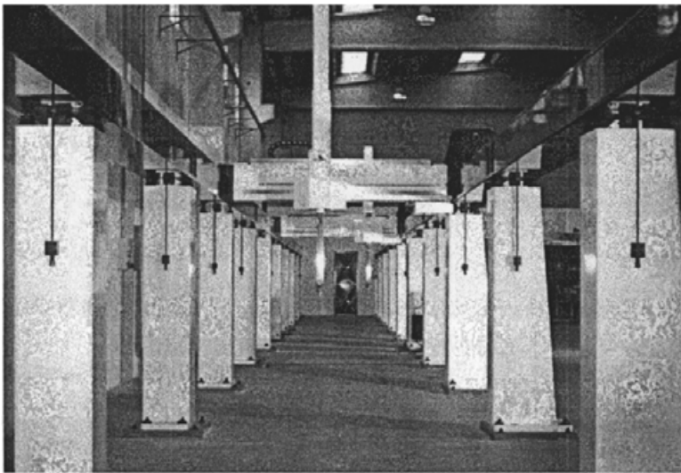
FIGURE 5.26 Automatic inspection station. (Courtesy Brown & Sharpe.)
