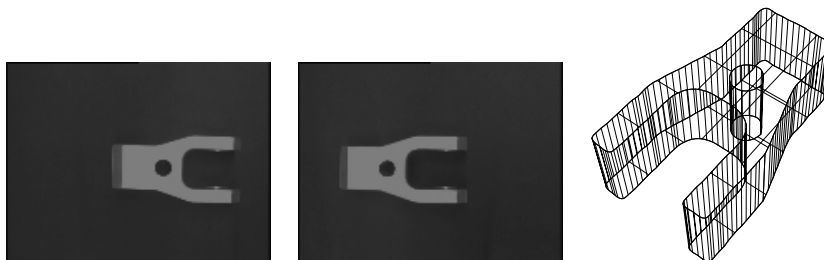
FIGURE 6.47 The two stereo images and the final \alpha_1 model that was found in the experiment.
