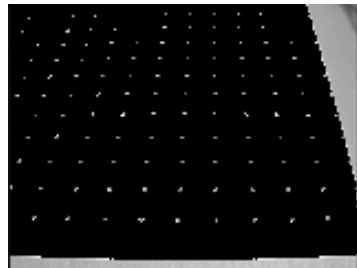
FIGURE 6.24 Thresholded calibration grid.
