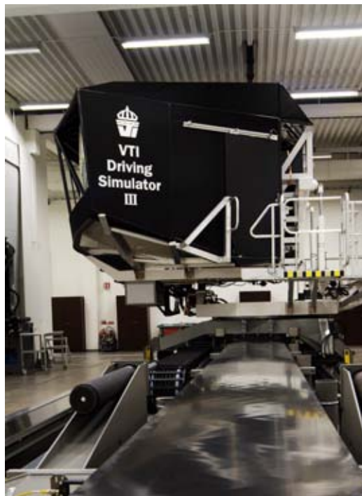
Figure 5.1 The motion system of the VTI Driving simulator III (Source: Swedish National Road and Transport Research Institute (VTI) (2004))
