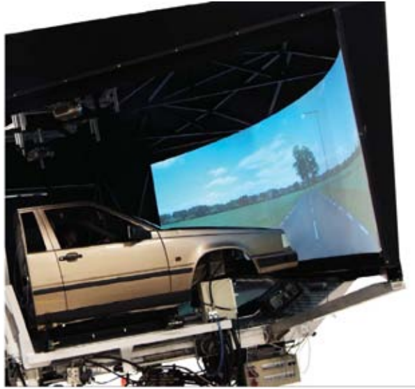
Figure 1.1 The VTI Driving Simulator III (Source: Swedish National Road and Transport Research Institute (VTI) (2004))
