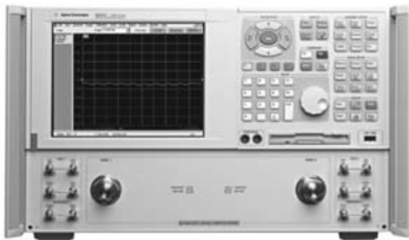
Figure 12.4 Modern vector network analyser covering the frequency range 10 MHz to 67 GHz
