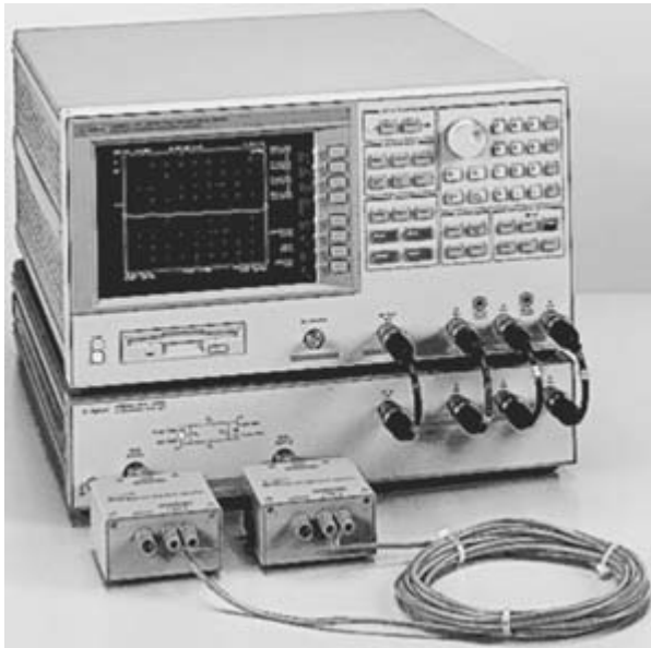
Figure 12.3 Network, spectrum, impedance analyser combined with a test-set used for making a wide range of RF and LF measurements
