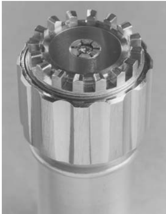
Figure 4B.1 The GR 900 14 mm connector [photograph NPL]
