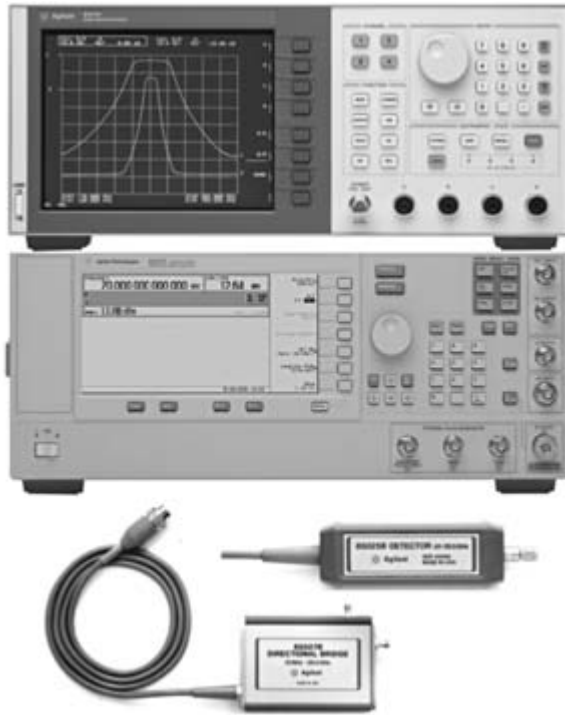
Figure 12.1 Photograph of a typical wideband detector based scalar network analyser and accessories
