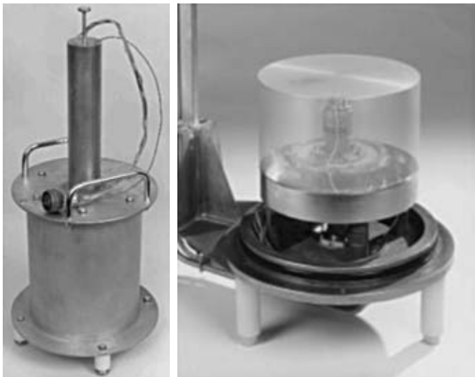
Figure 15.4 Waveguide calorimeters for WG27 and WG16
