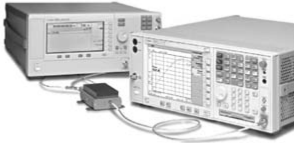
Figure 12.2 Photograph of a high-performance spectrum analyser based scalar network analyzer, which uses a high-performance external source as the tracking generator
