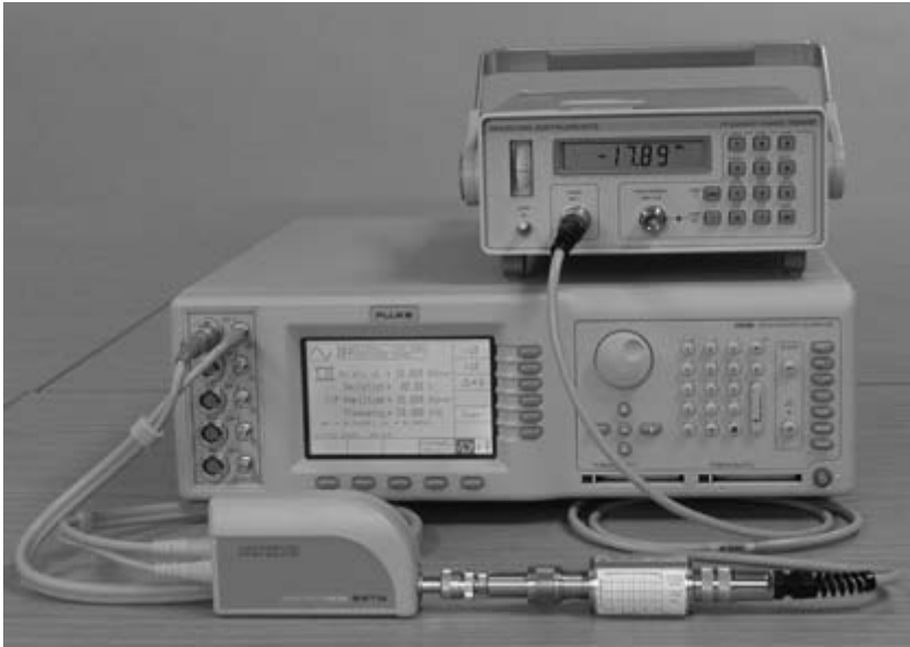
Figure 6.25 Photograph showing setup for levelled sine calibration up to 3.2 GHz against a power meter
