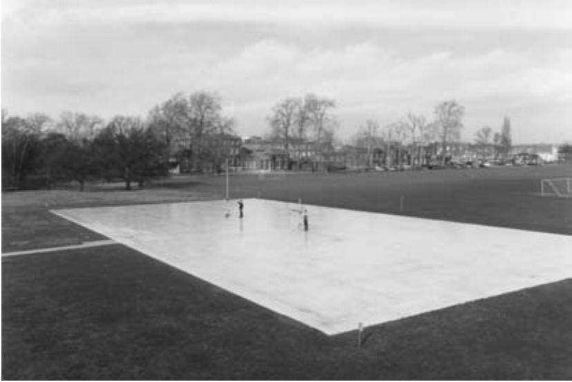
Figure 19.1 The 60 × 30 m ground plane at the National Physical Laboratory, Teddington, UK, whose surface is flat to within ±15 mm over 95 per cent of its area
