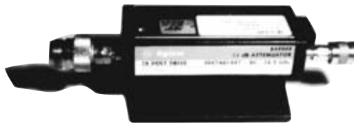
Figure 13.7 Artefact chosen for the comparison, an Agilent 84904K programmable step-attenuator with a type N adapter and short circuit fitted
