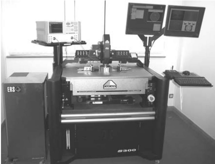
Figure 11.15 Photograph of the Summit S300-973 thermal probing system, capable of over temperature measurements from -65 to 200^{\circ}\text{C}
