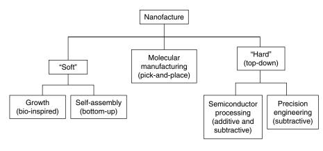
FIGURE 1.2 Different modes of nanomanufacture (nanofacture).
