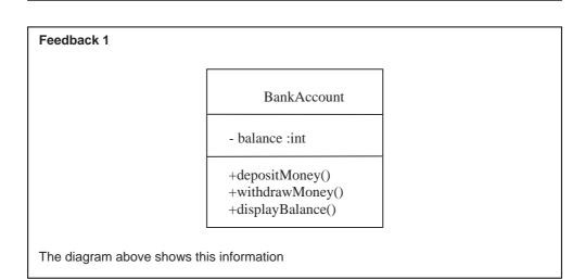
UML allows us to suppress any information we do not wish to highlight in our diagrams – this allows us to suppress irrelevant detail and bring to the readers attention just the information we wish to focus on. Therefore the following are all valid class diagrams...
