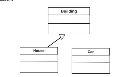
A house is a type of building and can therefore inherit the attributes of building however this is not true of a car. We cannot place two classes in an inheritance hierarchy unless we can use the term **is a**.
