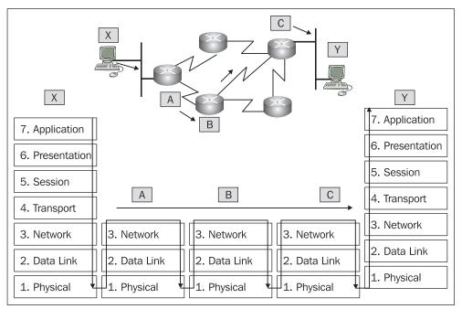
A packet originating from host X will get to host Y by traversing routers A, B, and C.
