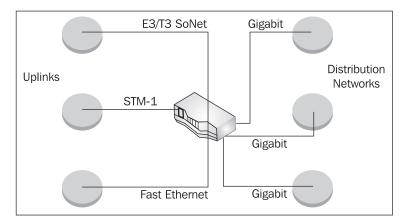
The router we had to choose had three uplink connections to other backbones of our network in a geographically distanced place. We rented an STM-1 connection from a carrier, an E3 connection from another carrier, and a FastEthernet connection from a third carrier. The router had to have three Gigabit connections to three distribution networks.
