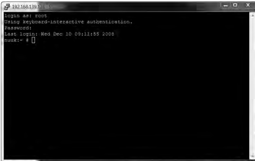
Figure 1-3. PuTTY is the de facto standard for accessing a Linux console remotely from a Windows workstation.
