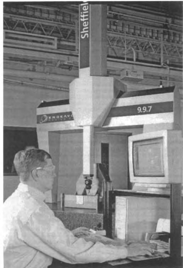
Fig. 14D1 Dimensional inspection of a machine component with a coordinate measuring machine. (Courtesy Sheffield Measurement, Inc.)
