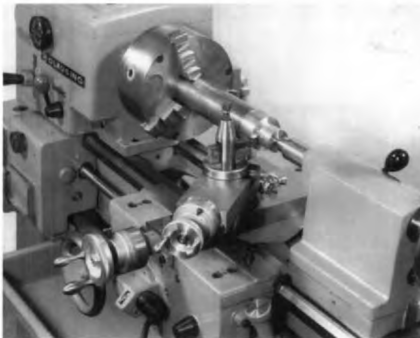
Fig. 3A2a A typical turning operation being performed on an engine lathe. The bar workpiece is held in the three-jaw chuck and is supported by a center in the tailstock. (Photo courtesy Clausing Industrial, Inc.)
