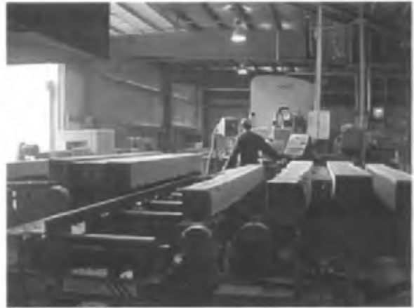
Fig. 6A3 Cants (squared logs) being cut into boards at a secondary saw. (Courtesy Connerstone Forest Products, Kingsley PA.)
