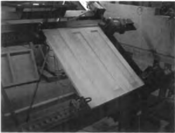
Fig. 6E1-2 Gluing fixture for assembly of cabinet doors. Pneumatic clamps provide pressure to seat all components and to square the assembly. The fixture can hold the panel assembly together until the glue sets, but most commonly is used only temporarily. After clamping, headless pins are driven into the panel to hold it together until the glue sets. (Courtesy Donald Dean and Sons, Inc., Montrose PA.)
