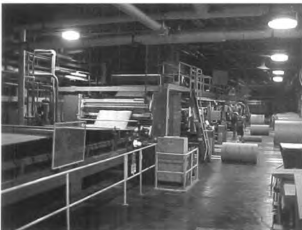
Fig. C4 A typical corrugating machine that makes either one or two layer boards, slits and cuts them to size for carton blanks and stacks the blanks for future use. The complete machine extends over 280 ft. (90 m) in length.
