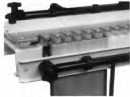
Fig. 6C6-1 Fixture for machining dovetail joints with a hand router. The dovetail cutter on the router follows the path controlled by the metal plate and machines both pieces to be joined in the same operation. Both pieces fit perfectly together with a line-to-line fit. (8 WMH Tool Group, Inc. All rights reserved.)
