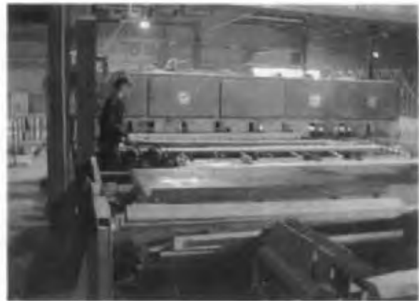
Fig. 6A7 The trimming operation with a multiple blade saw. The ends of the boards are trimmed square and defective or unfinished sections are removed at this saw. The operator determines, with computer assistance, for each board, where the cuts are made. (Courtesy Cornerstone Forest Products, Kingsley, PA.)
