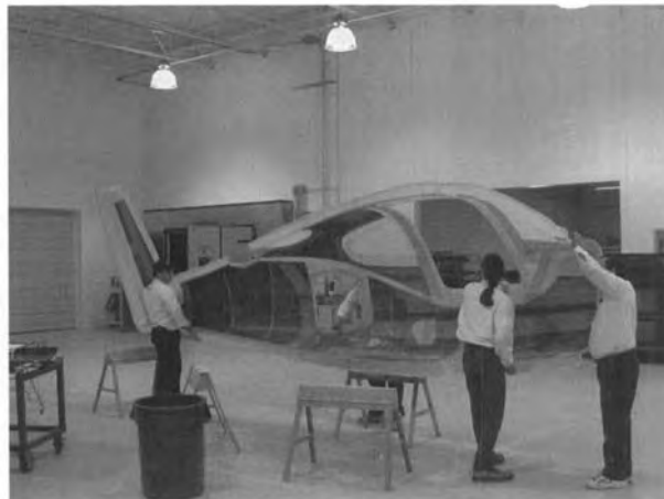
Fig. A6 One side of the major part of the cabin of a four-passenger private aircraft being moved into position for additional assembly. Note the light weight of the composite structure, permitting easy handling in the factory in addition to the flight advantages of such a structure. (Courtesy Cirrus Design Corporation.)
