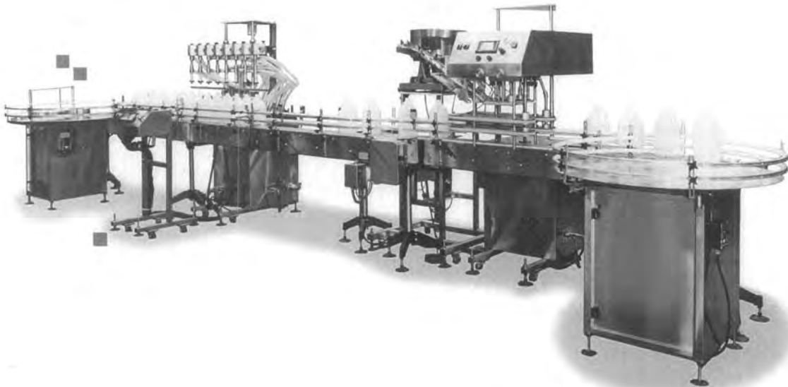
Fig. 12L A typical automatic bottling system. Bottles are fed to the line from the unscrambling table at the left where they are placed manually. They are conveyed to the filling station, where eight bottles are held and filled simultaneously. The bottles then are conveyed to the capping machine where caps are positioned and tightened, then to an accumulation table where they are removed and packed. Machines for larger production quantities may have automatic feeding and packing machines added to the system. Courtesy Inline Fillings Systems, Inc. , Venice FL.
