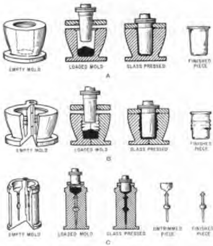
Fig. 5A2a Glass pressing with three mold variations: A - with a block mold, B - with a split mold, C - with a font mold. In C, excess glass on the part must be trimmed after pressing. (from Glass Engineering Handbook, E.B. Shand, McGraw-Hill, New York, 1958.)
