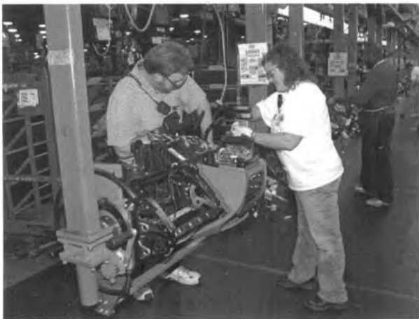
Fig. A9 A subassembly line for automotive dashboards. The fixture in the foreground holds the dashboard in an upside-down position, in which wire cable bundles, instruments, air bags, controls, a central console and other components are attached as the fixture moves along the line. Photo courtesy of General Motors.
