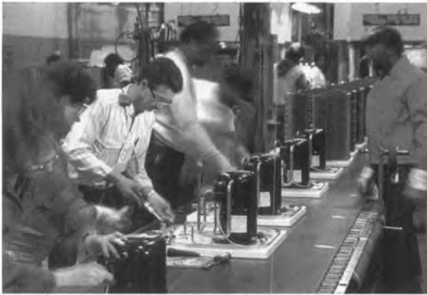
Fig. A2 An assembly line for the production of residential air conditioners. (Courtesy Carrier Corporation.)
