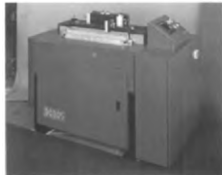
Fig. 6C6-3 This semi-automatic machine makes the dovetails of Fig. 6C6-2 with computer-numerical cutter control. The operator loads the two pieces to be joined. The machine cuts all the dovetails simultaneously, using as many of its 25 spindles as necessary. (Courtesy Dodds Co.)
