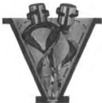
Fig. 11G3-2 A ribbon turbine with double spiral, for high-viscosity liquids. (Reproduced with permission from the McGraw-Hill Encyclopedia of Science and Technology, 1998.)
