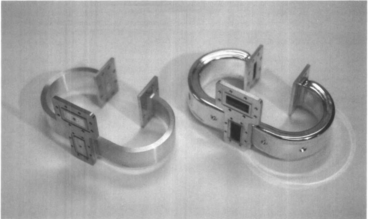
Fig. 2L2-1 A copper electroformed microwave guide (shown on the right) and the aluminum mandrel on which it was formed (shown on the left). The mandrel is dissolved chemically after the plated coating is of the desired thickness. The flanges in the finished part were "welded" to the guide by plating additional metal at the joint after assembly. Electroforming is particularly suitable for complex parts like this, particularly if surface details must be accurately produced. In this example, the interior dimensions are the most critical. (Courtesy A. J. Tuck Company)
