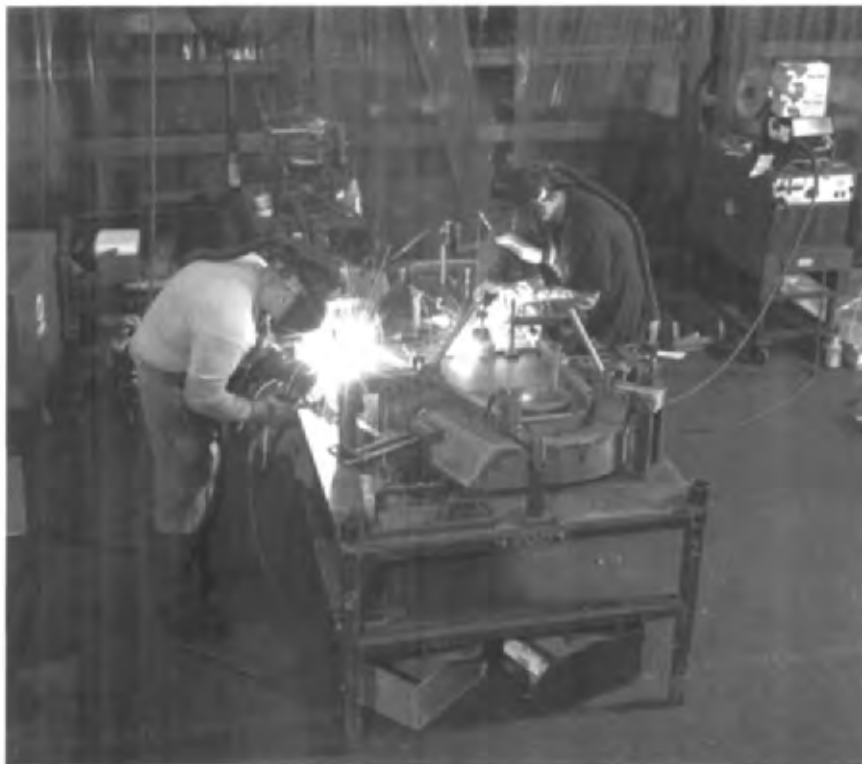
Fig. 7C1d-1 The production (GMAW) welding of the mower deck of a professional riding lawn mower. (Courtesy the Toro Company.)
