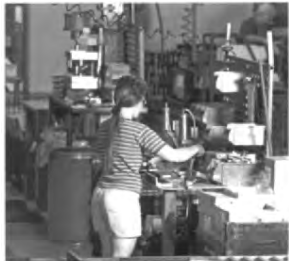
Fig. 7F1 Bench assembly. Note stacked bins for small parts, and devices mounted on the workbench for pressing component parts together. (Courtesy The Toro Company.)
