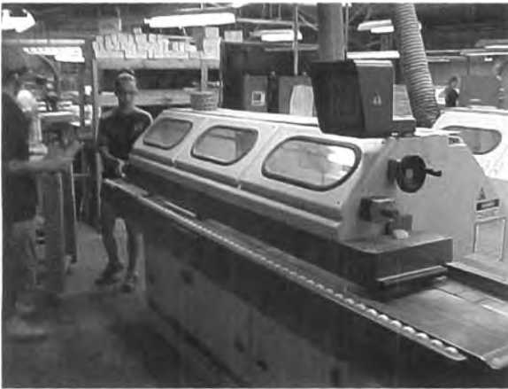
Fig. 6B7c A combination shaper and sanding machine that cuts a desired shape in the edge of the workpiece and then sands the area near the cut to remove burrs and sharp edges. (Courtesy Donald Dean and Sons, Inc., Montrose PA.)
