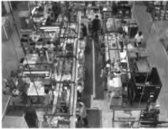
Fig. 7F2 An assembly line for the production of a powered hand tool. The operation starts at the workstation to the left of the painted line on the floor (near the bottom of the photograph). The line is U-shaped. As the assembly progresses, the product is handed from station to station and is complete when it reaches the last workstation on the right side of the painted line. There, it is packed in an individual carton. The worker at the base of the "U" (with his back to the camera) operates test equipment. This operation verifies the function, speed and safety of the tool. The operators off-line in the left side of the photo are doing bench subassembly of components that are incorporated into the product on the line. (Courtesy The Black and Decker Corporation.)
