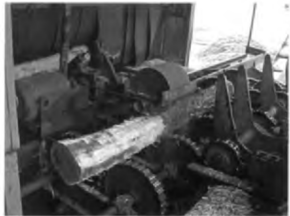
Fig. 6A1 A Rosser head debarking machine in operation. (Courtesy Connerstone Forest Products, Kingsley PA.)
