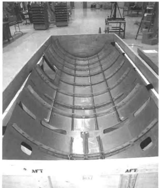
Fig. A4 Part of the cabin structure of a business jet aircraft. The stringers and ribs are fastened to the aluminum skin by friction stir welding (See 7C13i.) instead of with rivets. (Photo courtesy Eclipse Aviation.)
