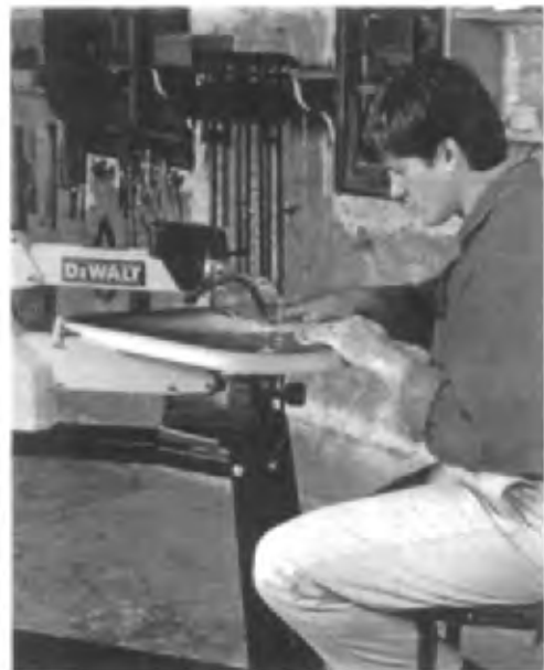
Fig. 6B3 A scroll saw is used for intricate decorative and other curved cuts in thin stock. (Courtesy DeWalt.)
