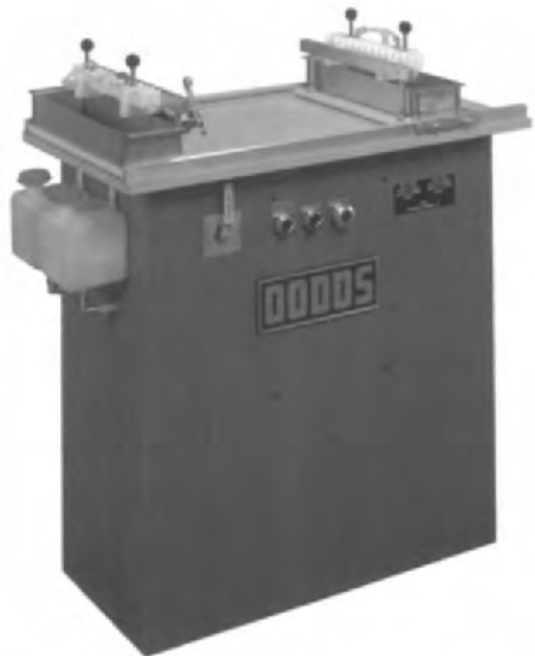
Fig. 6E3 A glue applicator machine for dovetail joints. When the board with dovetails is inserted, the machine dispenses a measured amount of glue from a manifold to each dovetail. (Courtesy DODDS Co.)
