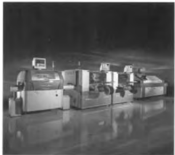
Fig. 13B2 An automatic assembly line for printed circuit boards with surface-mounted devices. All four machines are fully automatic, and the first three use machine vision to control the correct placement of parts and materials. The first of the four machines (at left) is a screen printer, which deposits solder paste on each pad that is to receive a lead from the devices to be assembled. The second and third machines pick and place circuit devices from paper or plastic tape fed from reels visible in front of the machines. The fourth machine is a convection reflow oven. It supplies heat with the proper heating profile to melt the solder paste, electrically connecting and mechanically fastening the devices to the board. (Courtesy Universal Instruments.)
