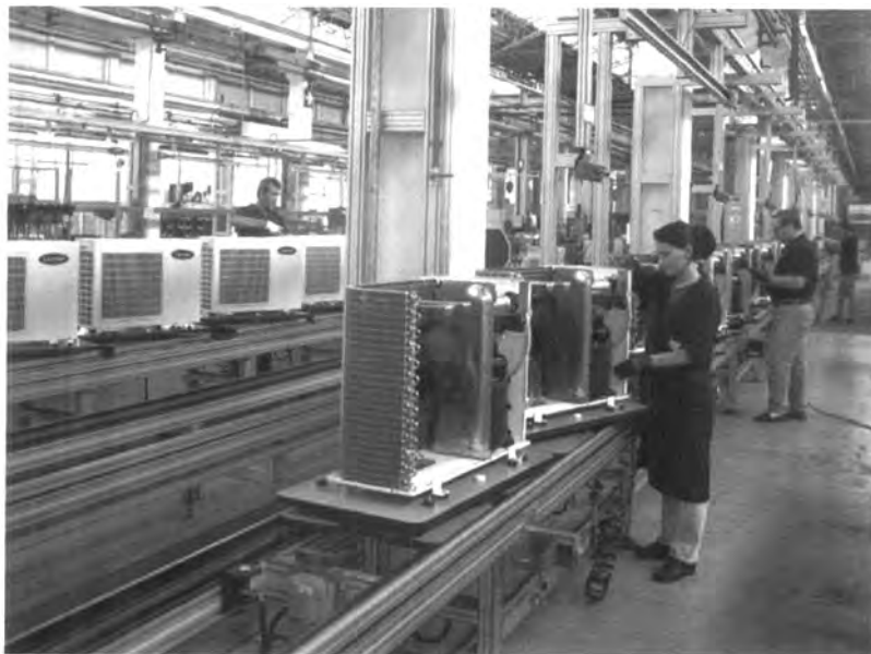
Fig. 7F2-2 A well engineered assembly line for the production of room air conditioners. (Courtesy Carrier Corporation.)
