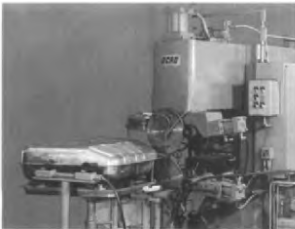
Fig. 7C6b Seam welding (RSEW) a vehicle fuel tank. (Photo courtesy Acro Automation Systems, Inc.)
