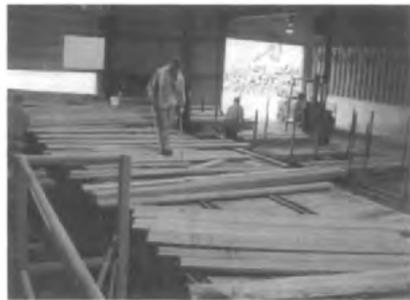
Fig. 6A8 Inspecting and grading green lumber. (Courtesy Cornerstone Forest Products, Kingsley, PA.)
