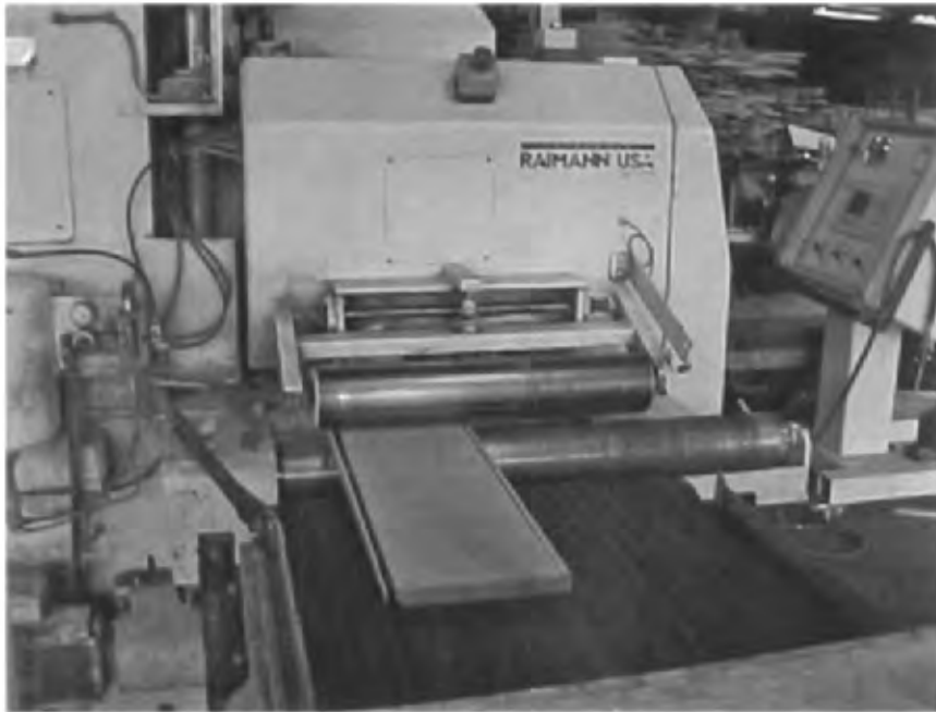
Fig. 6B1a Ripped boards exiting a multi-blade, computer-controlled, rip saw. (Computer functions are described in the text.) (Courtesy Donald Dean and Sons, Inc., Montrose, PA.)
