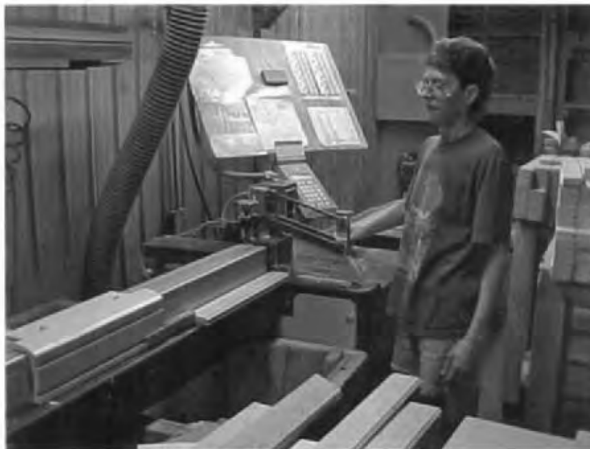
Fig. 6B1b-1 A chop saw. The operator keys in the workpiece length wanted in the key pad, and the machine then moves the work stop to the proper position. The circular cutting blade moves against the workpiece from underneath. (Courtesy Donald Dean and Sons, Inc., Montrose, PA.)
