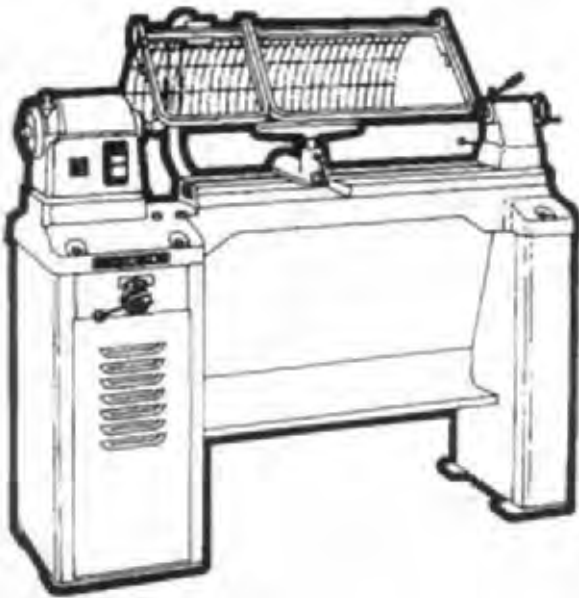
Fig. 6B4 A lathe for manually-controlled turning operations. (Courtesy Delta Machinery.)
