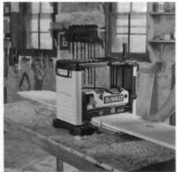
Fig. 6B2a-1 A planer used for craft work. (Courtesy DeWalt.)
