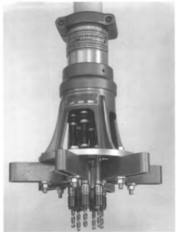
Fig. 3B8 A typical multiple spindle drilling head with provision for adjustment of the position of individual drills. (Courtesy RMT Technology, Bellwood, IL.)
