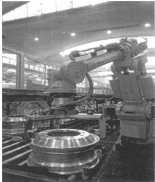
Fig. 14G12 Robotic handling of a large workpiece (an aluminum vehicle wheel) between machining operations. (Courtesy Alcoa Inc.)
