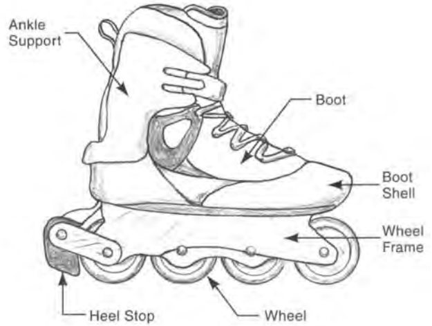
Fig. 11 The key components of typical in-line skates.
