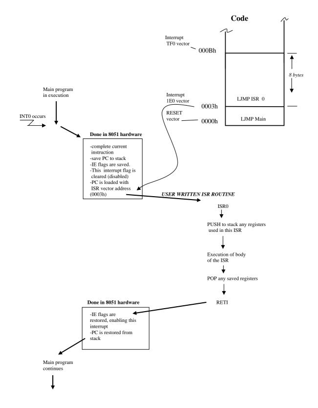
Figure 4.1 Interrupt operation example
