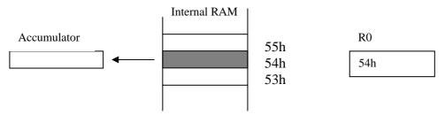
Note the @ symbol indicated that the indirect addressing mode is used. R0 contains a value, for example 54h, which is to be used as the address of the internal RAM
