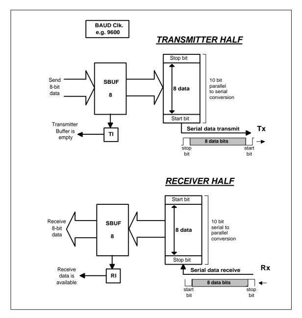
Figure 6.4 UART block diagram
