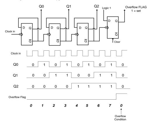
Figure 5.1 3-bit counter circuit
