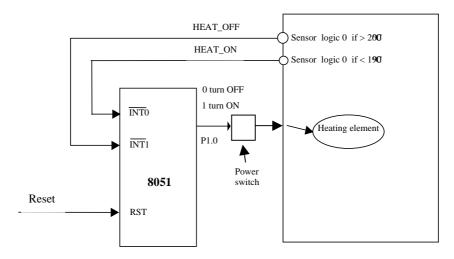
Figure 4.2 Temperature controlled heating oven
