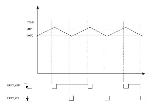
Figure 4.3 Timing diagram for the oven control
