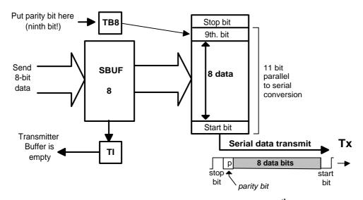
Figure 6.5 Block diagram of UART transmitter, using the 9<sup>th</sup>. bit
