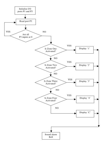
Figure 2.3 ALARM\_2 Program flow chart
