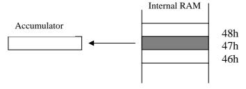
The instruction reads the data from Internal RAM address 47h and stores this in the accumulator. Direct addressing can be used to access Internal RAM, including the SFR registers.
