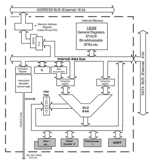
Figure 1.4 8051 showing the on-chip I/O devices
