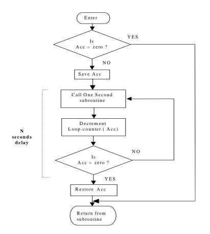
Figure 3.3 PROG\_DELAY\_SUB flow chart
