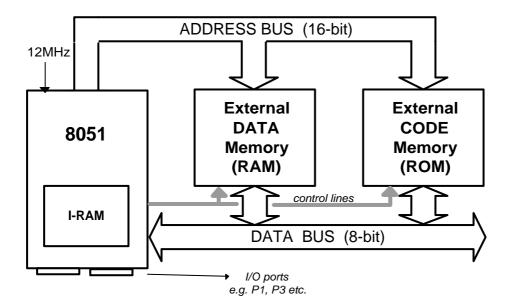
Figure 1.2 8051 chip with external memory
