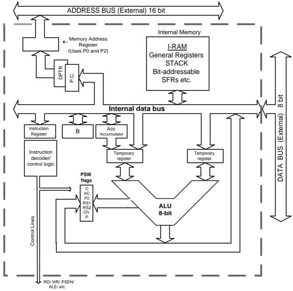
Figure 1.1 8051 functional block diagram.
