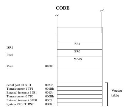
Figure 4.4 Code positioning in code memory space
