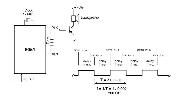
Figure 3.4 Hardware circuit with timing diagram
