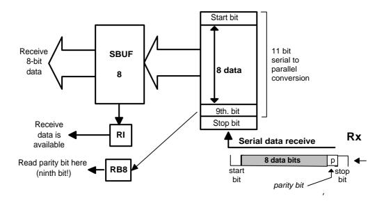
Figure 6.6 Block diagram of UART receiver, using the 9<sup>th</sup>. bit
