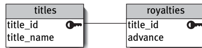
Figure 2.11 This diagram shows an alternative way to depict the one-to-one relationship in Figure 2.10. The connecting line indicates associated columns. The key symbol indicates a primary key.
