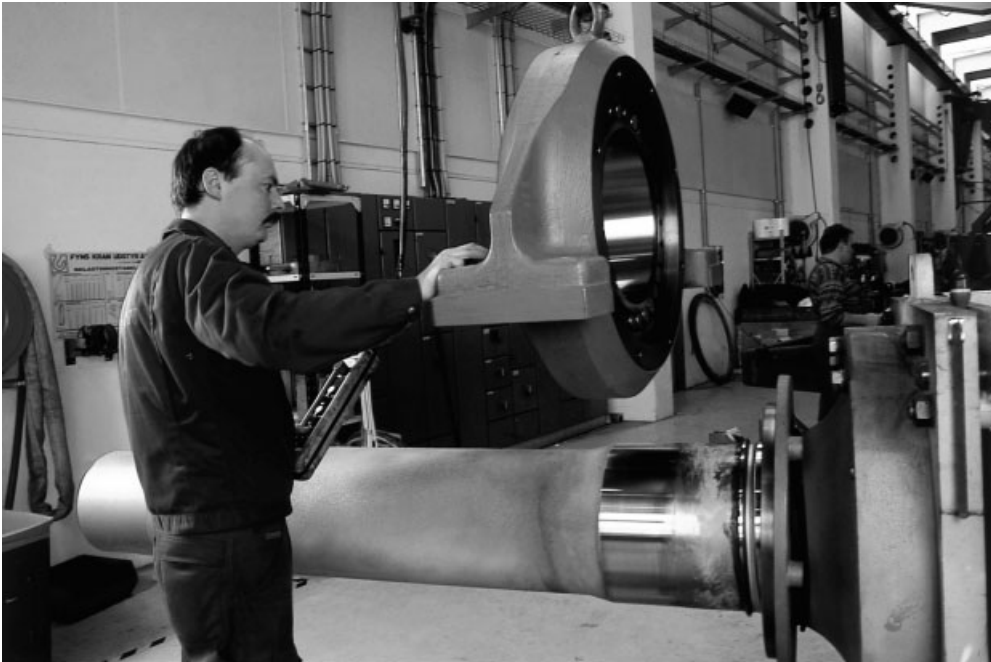
Figure 5.39 Low-speed Shaft and Front Bearing Before Assembly. The hub mounting flange at the right-hand end is bolted to a temporary support to allow the bearing to be threaded on the shaft. (Reproduced by permission of NEG Micon)
