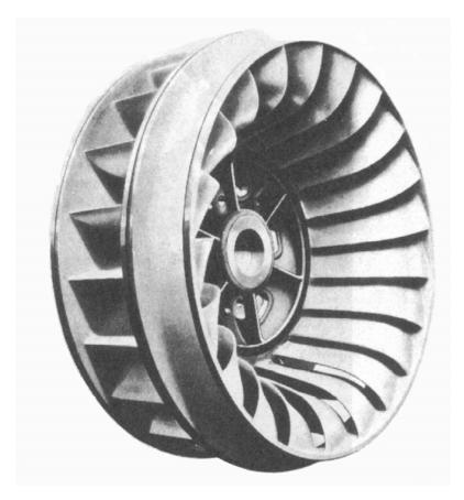
Fig. 5.50 Francis runner at Niagara Falls. Diameter = 176 in, H = 214 ft, N = 107 rpm
