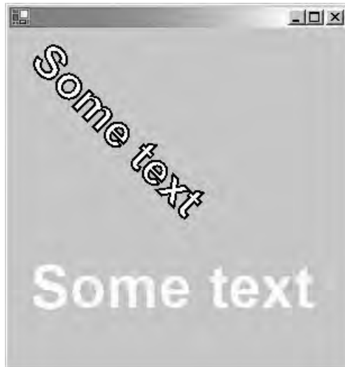
Figure 10.21 Text outline drawn with a Pen for the outline and a Brush for the interior
