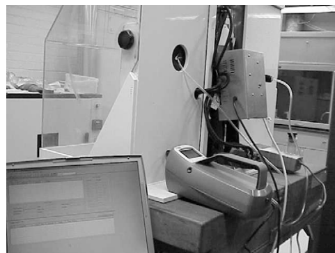
FIGURE 9.4 Pilot set-up involving both CPC and laser particle counter.
