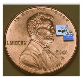
Figure 6. Smart mote on a U.S. penny (Kahn & Warnecke, 2006)
