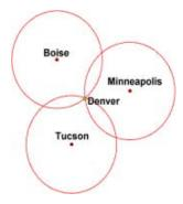
GPS is enabled by a constellation of 27 earth-orbiting satellites, 24 of which are in active operation at any one time. Each satellite circles the globe twice a day with orbits arranged so that at any time, anywhere on earth, there are at least four satellites "visible" in the sky. A GPS receiver is a device that locates at least three satellites to determine its distance to each and use this information to deduce its own location (Anonymous 1, 2007; Brain & Harris, 2007).
