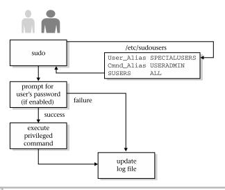
Figure 7-3 High-level function of sudo
