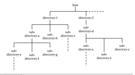
**Figure 6-2** Tree structure of a file system
