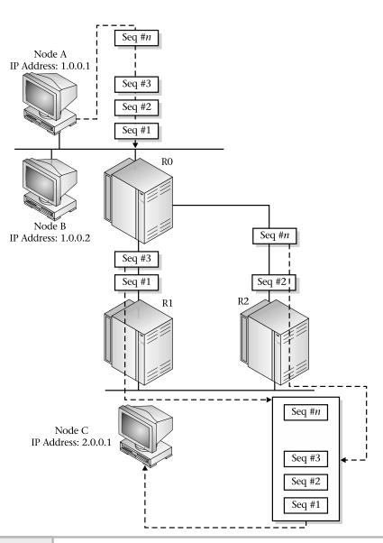
**Figure 10-3** TCP sequence numbers in action
