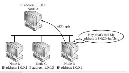
**Figure 10-18** ARP reply example
