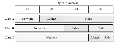
Figure 10-11 IP network classes with subnets addressing
