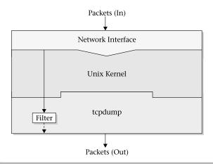
Figure 12-1 Packet filter diagram
