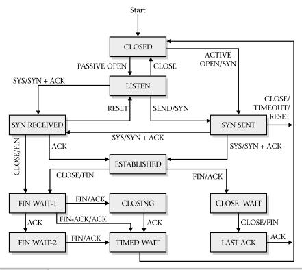
Figure 10-8 TCP state machine diagram
