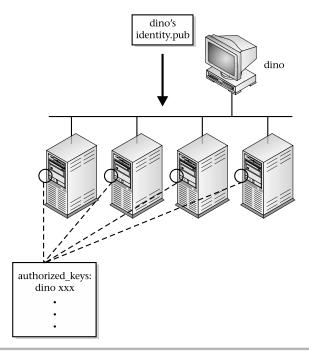
Figure 7-2 SSH host key placement
