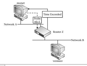
**Figure 12-2** Using traceroute with single hop in network
