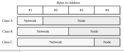
**Figure 10-10** Three primary IP address classes
