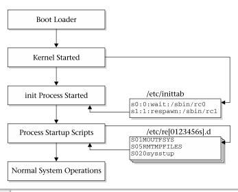
Figure 9-1 UNIX boot process
