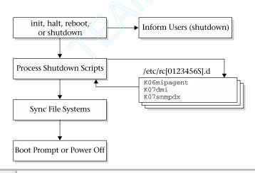
**Figure 9-2** UNIX shutdown process
