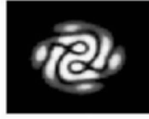
Fig. 3.1. Numerical calculation of the pattern generated by a frequency-degenerate OPO operating in a detuned quasi-confocal cavity ( \delta_s = -1.5\kappa , \xi = 0.25\kappa ), 70 times above threshold, and with a strongly focused pump field ( w_{pump} = 0.25w_0 ).
