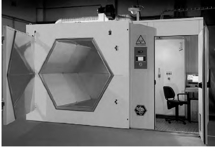
FIGURE 5.9 A large microwave cavity for uniform heating in batch industrial applications. The large size compared to the wavelength at 2450MHz ensures launching a large number of modes that contribute to heating uniformity. Multiple source, multiple feed points at total power level up to 30kW also contribute to uniformity and high energy deposition intensity. (Courtesy of Vötsch Industrietechnik GmbH; the unit is commercially marketed as the Hephaistos System. After Ref. [26].)
