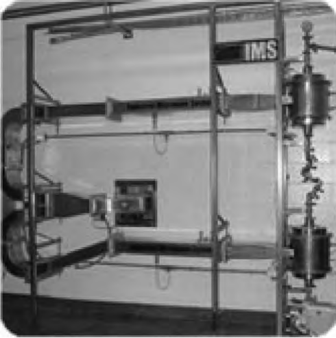
FIGURE 4.14 A two-stage single-mode cavity heating installation for microwave processing of fluids. (Courtesy of Industrial Microwave Systems (IMS).)
