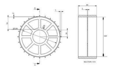
Figure 3 2D Drawing of Rover Wheel
