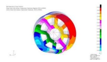
Figure 8 Alumminium Displacement Plot Maximum displacement=0.0213mm
