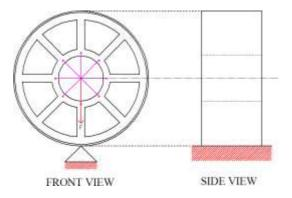
Figure 7 Impact Load Boundary Conditions Plot
