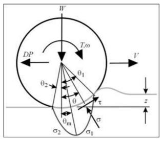
Figure 4 Diagram of Wheel/Soil Interactions
