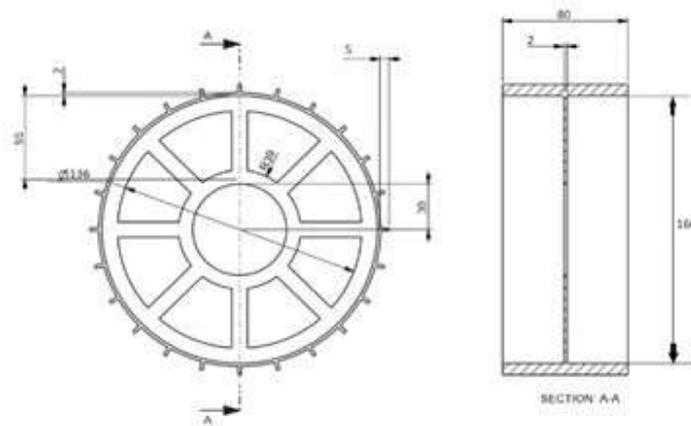
**Figure 3** 2D Drawing of Rover Wheel
