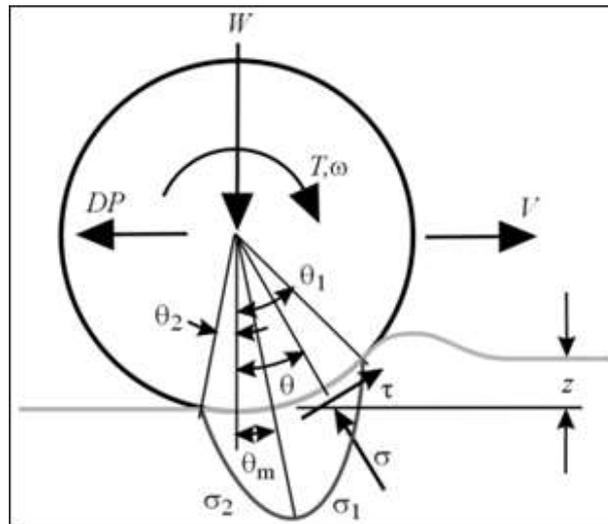
Figure 4 Diagram of Wheel/Soil Interactions
