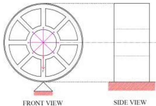
**Figure 7** Impact Load Boundary Conditions Plot
