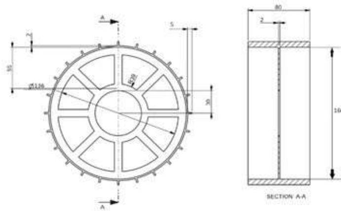
**Figure 3** 2D Drawing of Rover Wheel
