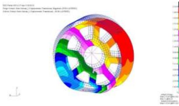
**Figure 8** Aluminium Displacement Plot Maximum displacement=0.0213mm
