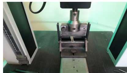
Fig. 4. Shows UTM with flexural specimen
