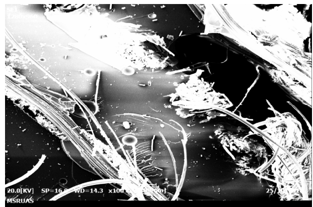
Fig. 11. Shows tensile fracture of hybrid composites using hand lay up technique
