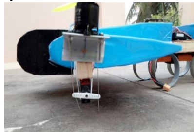
Figure 6 : Parallelogram four bar Mechanism
