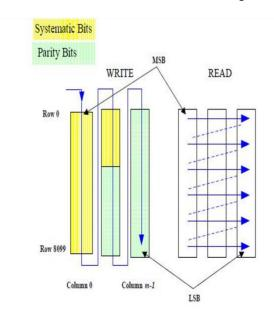
Fig 2: Row-column interleaver
