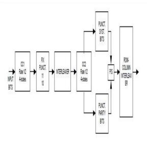
Fig.1: Block diagram of SCCC scheme
