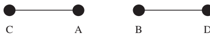
Figure 5.9 Neighboring nodes A and B have different schedules. They synchronize with nodes C and D respectively.
