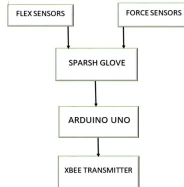
Fig. 1: The Sparsh Glove Block Diagram
