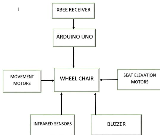
Fig 4: Wheelchair Block Diagram.
